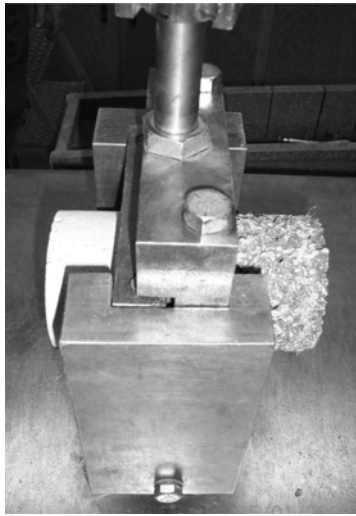
Fig. 6—Overlay bond strength test setup.
